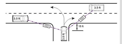
Intersection sight distance (ISD) measures a line of sight from the height of driver's eye (3.5 feet), seated 15 feet back from the fog line or edge of the traveled way, to the right and to the left, to an object in the highway that is 3.5 feet high.
