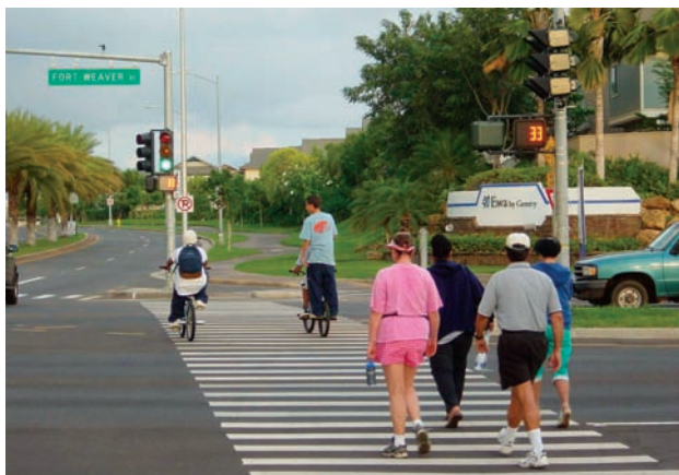
Pedestrian signal head in line with crosswalk
