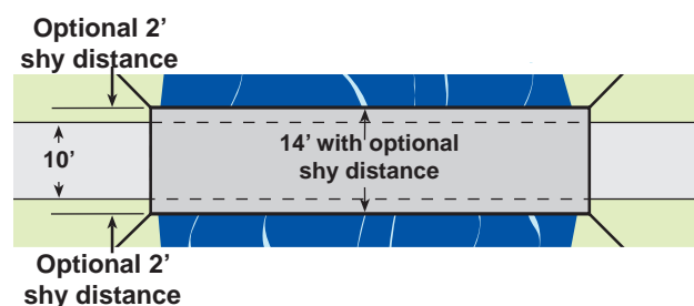
Figure 7-13: 14 feet wide bridge serves a 10 feet wide path
