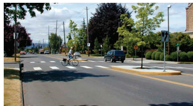
Road diet created room for median pedestrian refuge island
