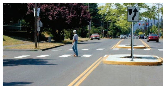
Median island provides mid-street refuge for pedestrians
