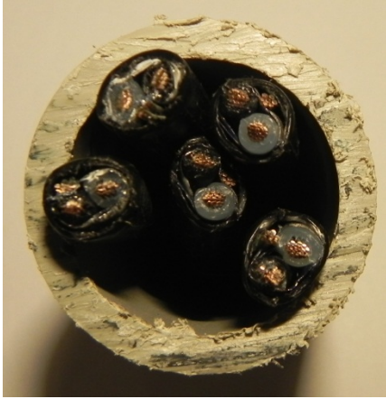
1" conduit w/5 loop feeder cables Exceeds NEC max fill Exceeds ODOT max fill
