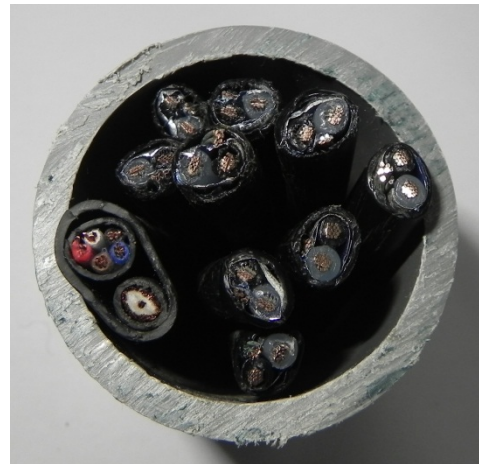
1 1/2" conduit w/9 loop feeder cables +1 video cable Exceeds NEC max fill Exceeds ODOT max fill
