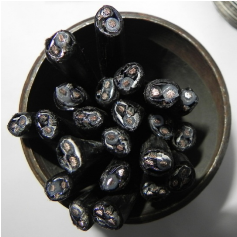
2½" conduit w/22 loop feeder cables Exceeds NEC max fill Exceeds ODOT max fill
