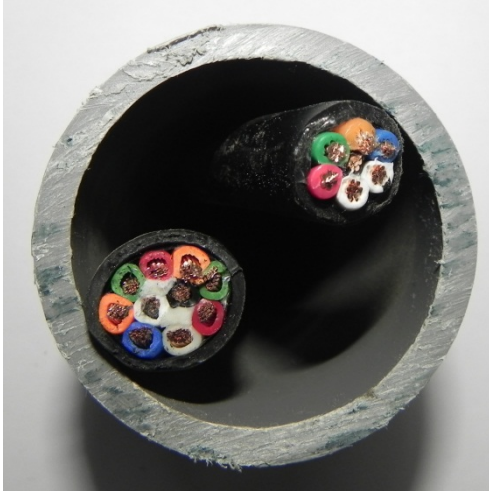
1 1/2" conduit w/control cables Does NOT exceed NEC max fill Does exceed ODOT max fill
