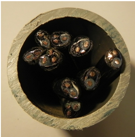
1 1/2" conduit w/9 loop feeder cables Does NOT exceed NEC max fill Does exceed ODOT max fill
