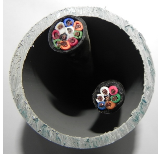
2" conduit w/control cables Does NOT exceed NEC max fill Does NOT exceed ODOT max fill
