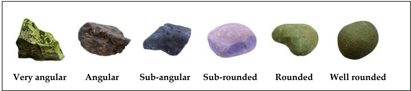
Figure 5-5 Particle Shape for Coarse-Grained Soil Particles
