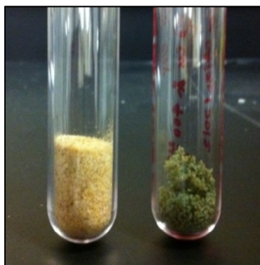
Figure 4.20: Sieved Apatite II™ before (left) and after (right) a column experiment
