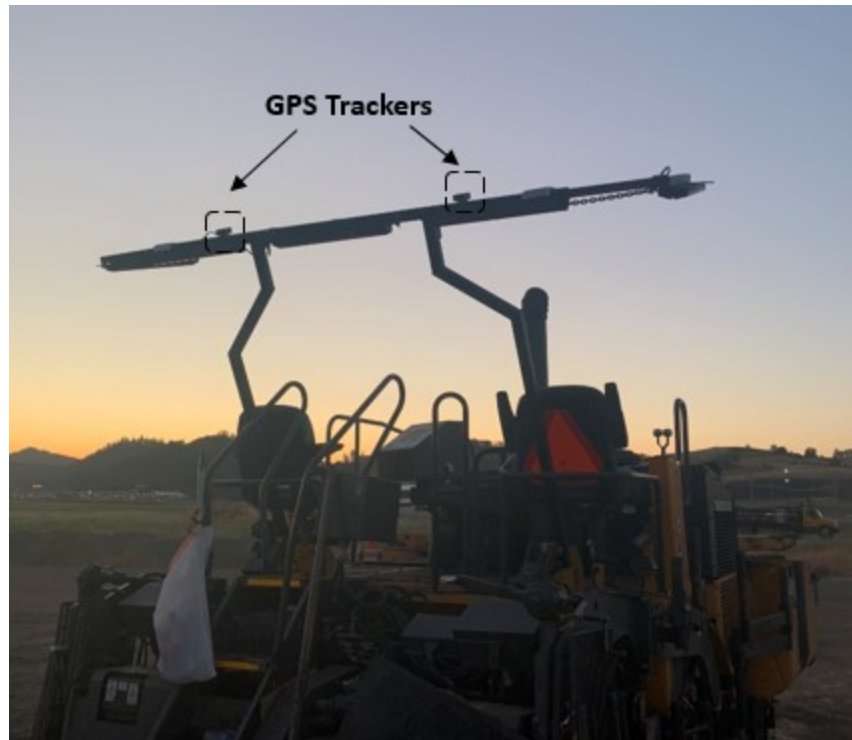
Figure 5.8: GPS trackers placed on a paver
