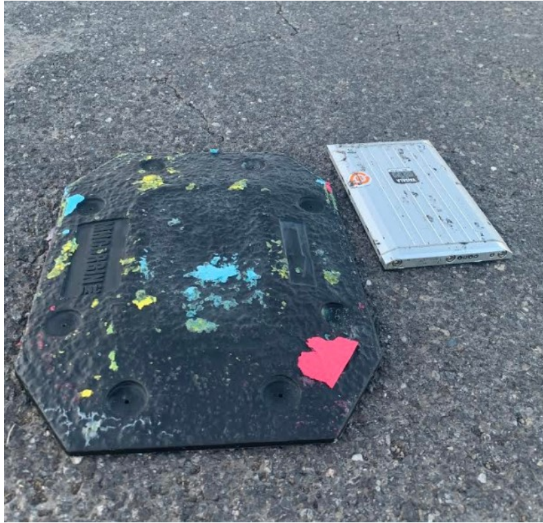
Figure 5.1: Portable traffic analyzer components: Cover (left) and analyzer (right)
