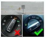
In addition, daytime running lights (DRL) on most new vehicles may activate white lights to the front but leave the taillights off which leads to many driving at night or in inclement weather feeling headlights are on without any rear lighting being present. If in doubt, turn your headlights on.
