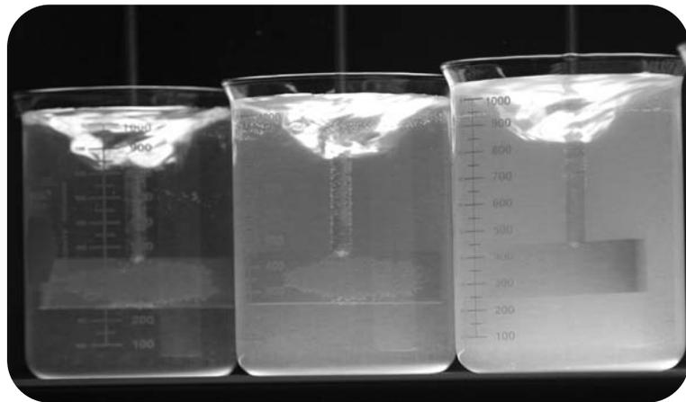
stirrers to match the conditions in the flocculator and allow them to operate for 30 minutes. Observe the floc formation periodically during the 30 minutes. At the end of the 30 minutes turn off the stirrers and allow settling. Most of the settling will be complete after one hour.
