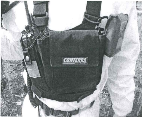
Pictured below is the Canberra Ultraradiac personal radiation monitor. Designed to electronically alarm when personnel are in high levels radiation areas
