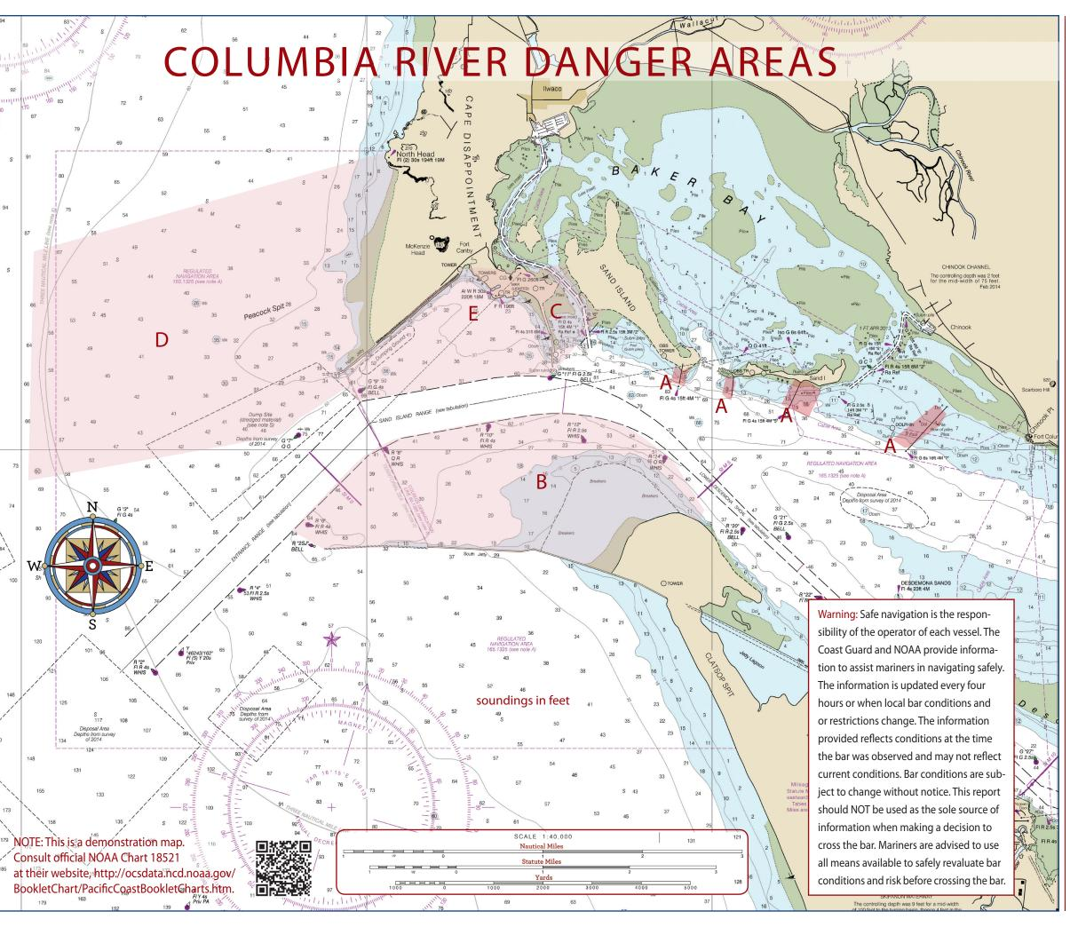
A. Chinook spur and upper, lower, and middle Sand Island spurs are built on two rows of staggered pilings. Currents flowing through these pilings attain a velocity of five knots or more. A boat that becomes disabled or is maneuvered in such a way that it comes in contact with any of these spurs is almost sure to suffer damage. Even large boats have capsized in these areas. Give these spurs a wide berth and never get close to them on the up-current side.
