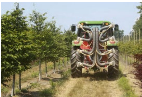
Airblast sprayer, photo by the Hood River Soil and Water Conservation District.
