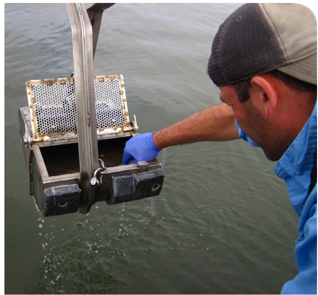
Image 14: Lowering an Eckman Dredge to collect benthic samples for the National Coastal Condition survey. Harney
