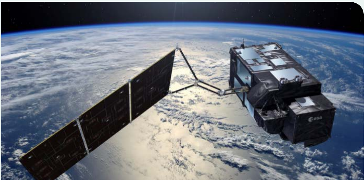
Image 7: This earth observation satellite has an Ocean Land Color Instrument or OLCI is for used to monitor harmful algae blooms in Oregon.
