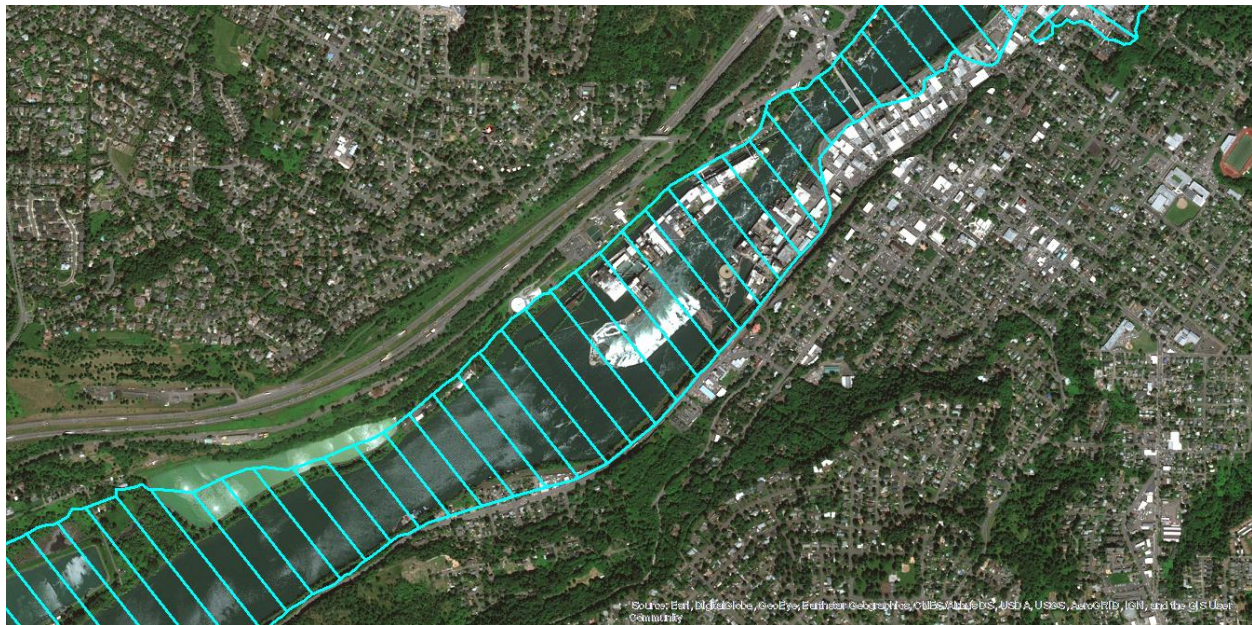
Figure 3-29 Example of 100-meter wide floodplain survey “slices” within a 1mi long reach in the Willamette Falls area (RM 26.7). Data source: http://ise.uoregon.edu/slices/data.html
