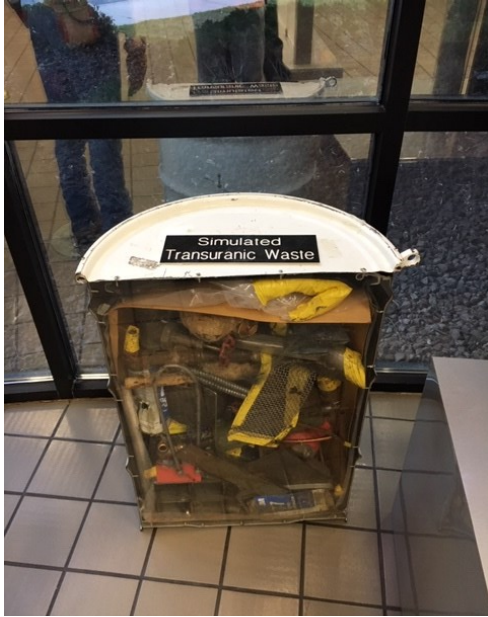
TRU container with contaminated equipment.
