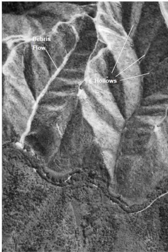
Figure 4a. Aerial View of a High Density of Bedrock Hollows in the Central Oregon Coast Range. This photograph also shows a landslide in a bedrock hollow, triggered by a logging road, that transformed into a debris flow that deposited sediment into a larger stream. Source: Benda, Lee, Curt Veldhuisen, Dan Miller, Lynne Rodgers Miller. 1998. Slope Instability and Forest Land Managers – A Primer and Field Guide . Earth Systems Institute
