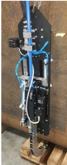
Magnetic wheeled air slot visual inspection crawler
