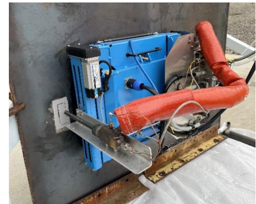
Cold-spray patch testing
