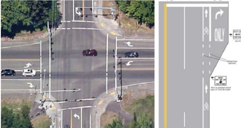
Figure 3-5. Right-turn Lane on Both Major Road Approaches
