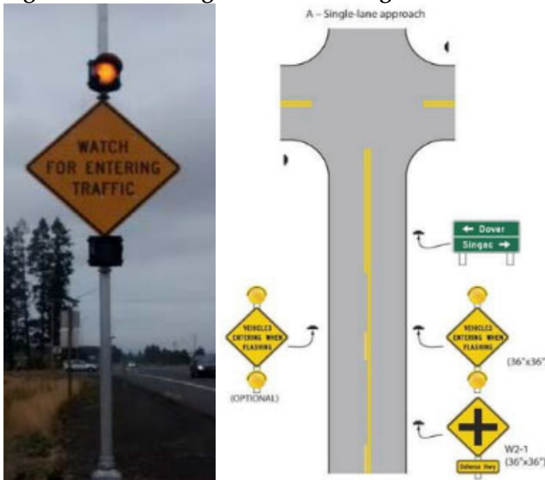
Figure 4-26. Flashing Beacons at Unsignalized Intersection
