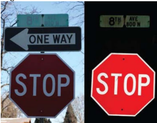
Figure 4-23. Retroreflective Stop Sign in Daylight and Nighttime Conditions
