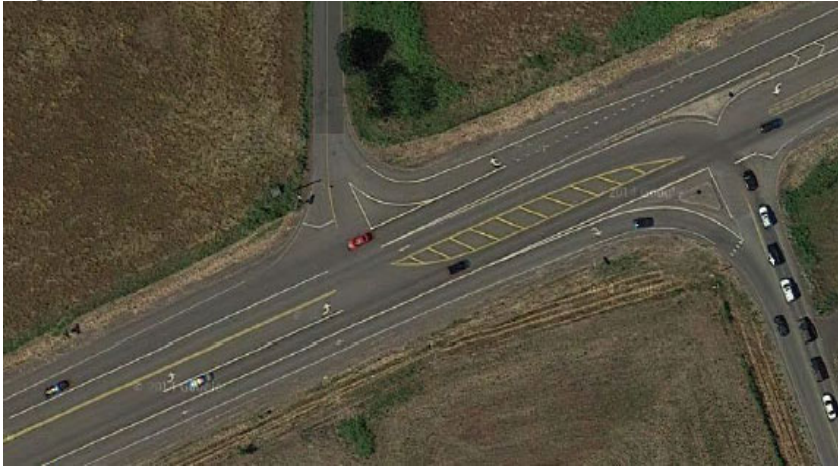
Figure 3-28. Median Acceleration Lane
