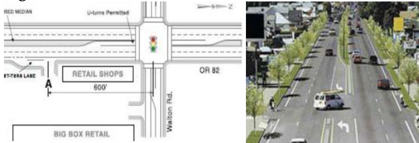
Figure 3-38. Raised Median on Urban Multilane Road
