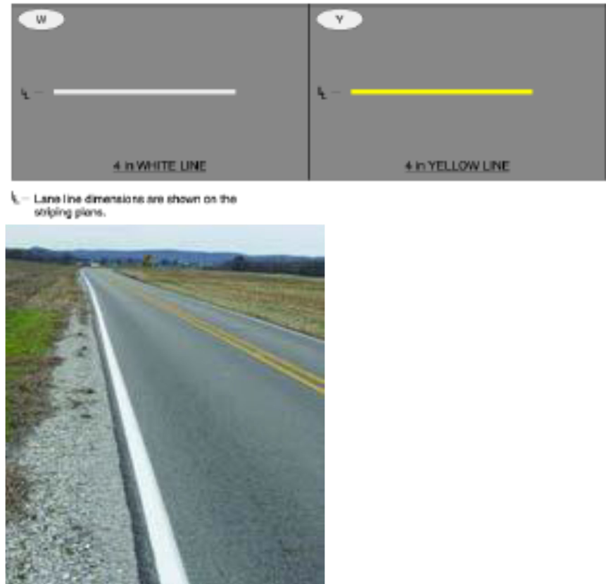
Figure 6-15. Edge Line for Rural Roadways
