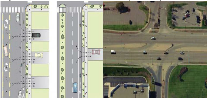
Figure 3-36. Reduce Urban Driveway Density
