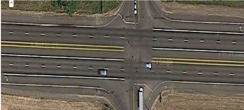
Figure 3-3. Right-turn Lane on Both Major Road Approaches
