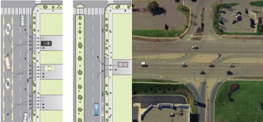
Figure 3-35. Reduce Urban Driveway Density
