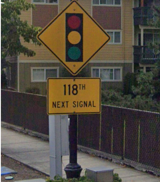
Figure 4-22. Signal Ahead Sign
