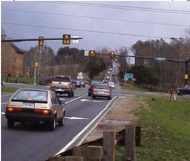
Figure 4-7. Intersection Traffic Signals Converted from Nighttime Flash Mode to Normal Steady Operation
