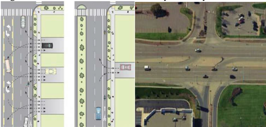
Figure 3-34. Reduce Urban Driveway Density
