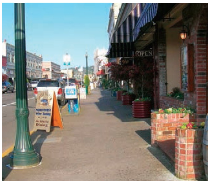
Figure 800-12: Sidewalk with a Clear Pedestrian Zone
