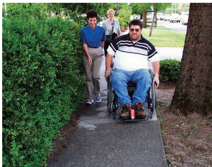
Figure 800-13: 5-Foot Sidewalk is Uncomfortably Narrow
