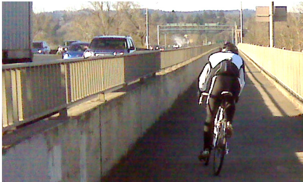
Figure 900-14: Concrete barrier as street buffer
