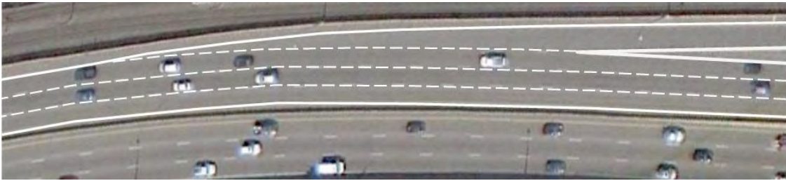
Figure 4-1: Typical Freeway Entrance Ramp Merge Area
