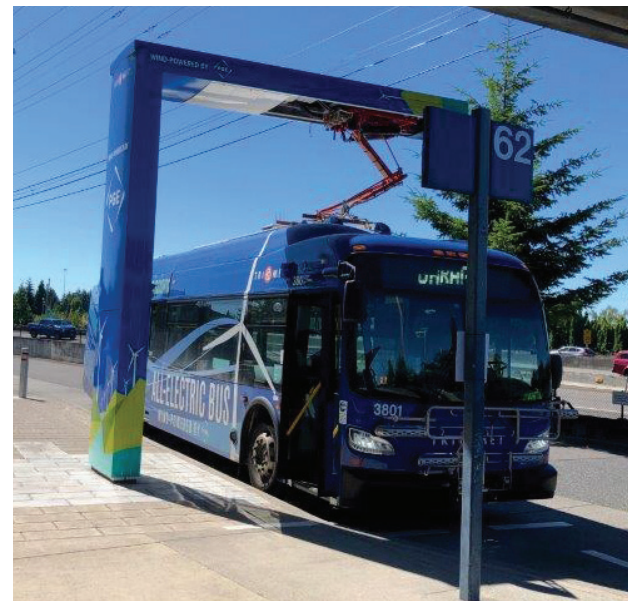
TriMet electric bus using overhead pantograph charging at a stop along its route.
