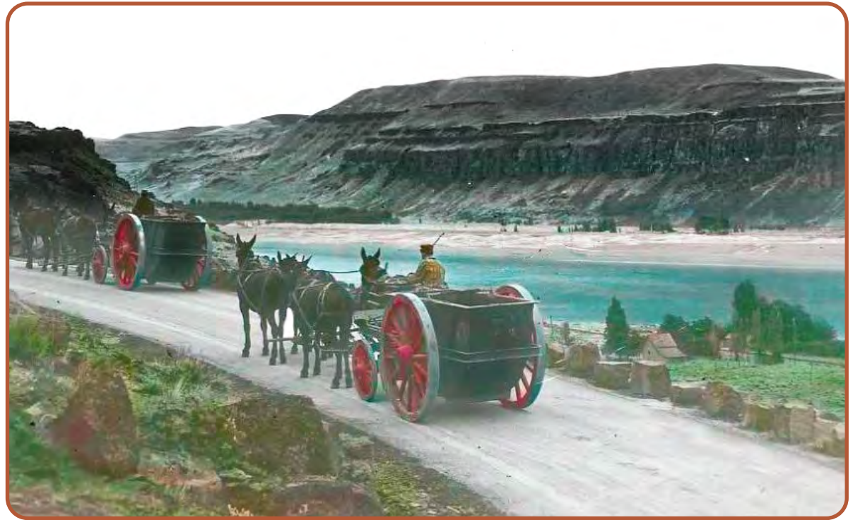
EXHIBIT 5: Steel road construction wagons designed by Samuel Lancaster. Photo: Maryhill Museum of Art.
