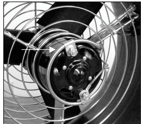
Flow Sensor on Duct Blaster Fan
