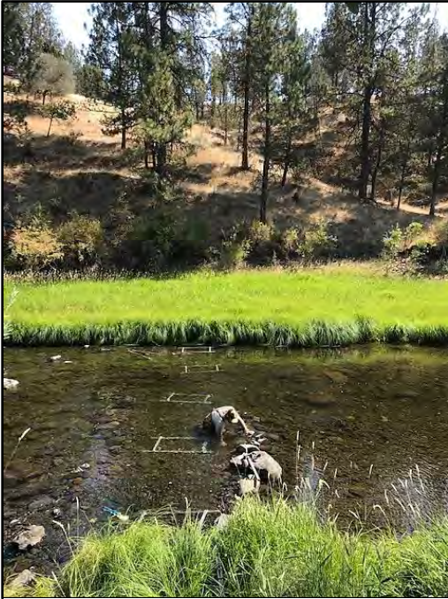
Figure 7. Installation of a channel spanning PIT-tag array near Ritter, at the downstream end of fish monitoring in the MFJD. Photo Credit: ODFW
