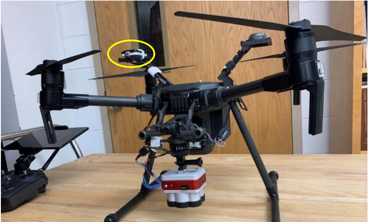
Figure 1: Matrice 200 with Altum Multispectral Sensor – yellow circle identifies incident light sensor
