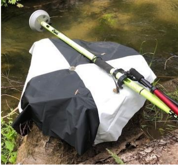
Figure 4: Iron Cross aerial survey target
