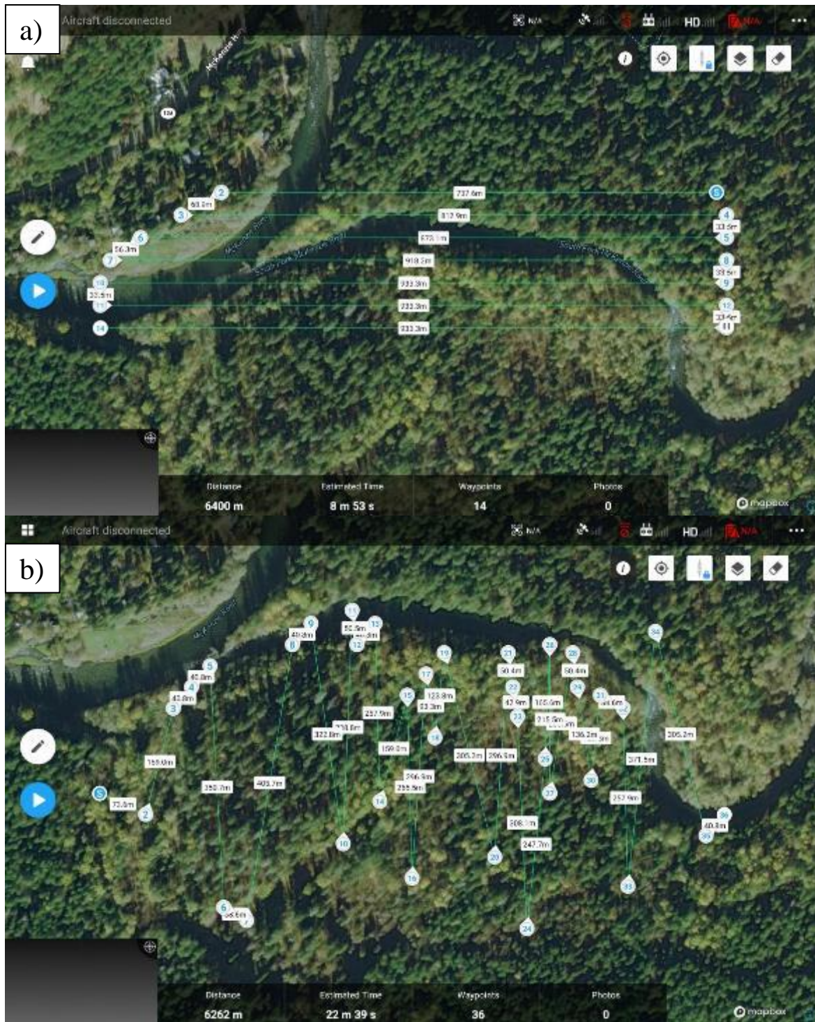
Figure 5: Flight profiles. a) Aerial survey profile over Phase I as viewed in the DJI GS Pro application. b) Overview of the Photo/video plot profile in the DJI GS Pro application.
