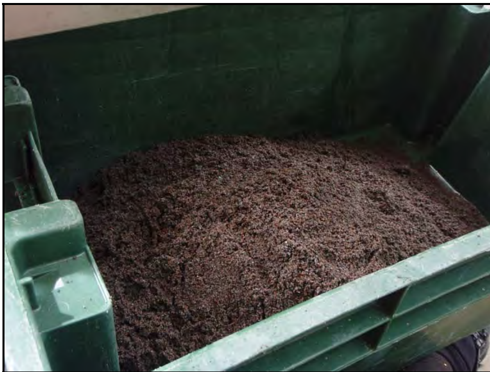
Figure 3-14. Bedload sample collected at 5,000 cfs on May 15, 2008 (#2008-20).
