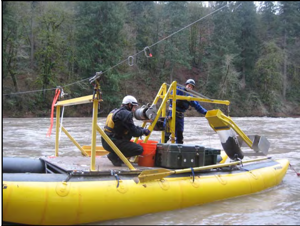
Figure 3-13. TR-2 bedload sampler nearly filled with sand after two verticals at 5 seconds.
