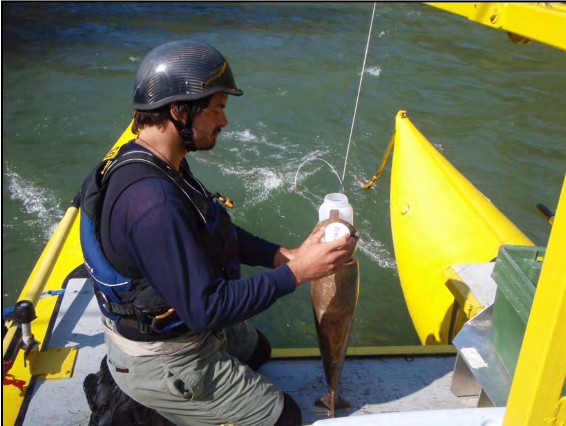
Figure 2-3. Loading the D-74 suspended sediment sampler with a quart sample bottle.
