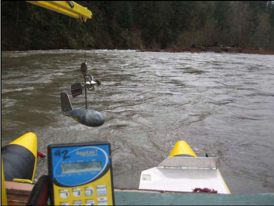
Figure 2-2. Price AA current meter on a 100 lb sounding weight deployed from a cataraft.
