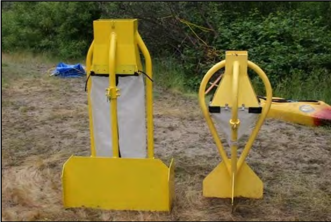
Figure 2-4. The TR-2 (left) versus the 6 inch Helley –Smith bedload sampler.
