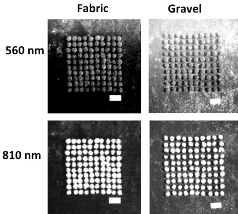
Multispectral imagery at 560 and 810 nm that can potentially be utilized for improved counting accuracy.
