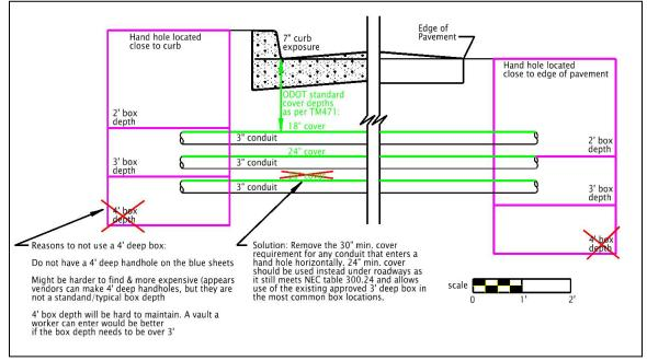
Changed minimum dimension of softscape from the edge of sidewalk or edge or ramp from 3 feet to 2 feet in "Junction box installation in unsurfaced area" detail
