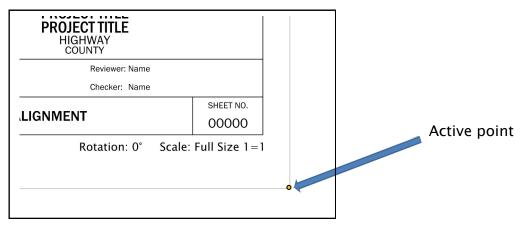
*Step 5*: In each of the models for the specific sheet series, the title block text cells have been placed. If each plan sheet has unique text, delete the text cell from the series model and place the text cell inside the sheet file. Another cell is outside of the title block border that lists the numbered levels that the approved sheet titles are on. The model for the N series plans does not have this cell.
