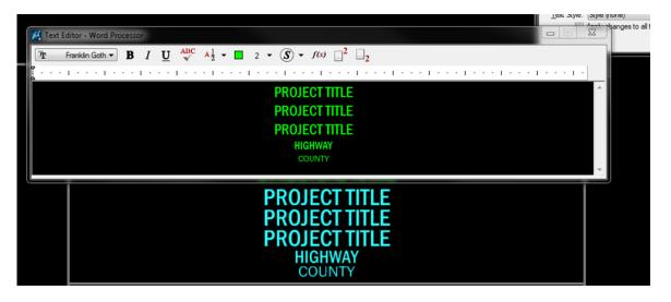
Selecting all the text "PROJECT TITLE" a single line can be edited to the text node. Longer project names need to be spaced such that they have a pleasing appearance in the space provided. The highway name is edited onto the line with the default text "HIGHWAY" and the county name is edited onto the line with the default text "COUNTY".
