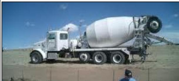
The third SHV model is the SU6, which is a six axle vehicle with a gross vehicle weight of 69,500 LBS (34.75 tons).
