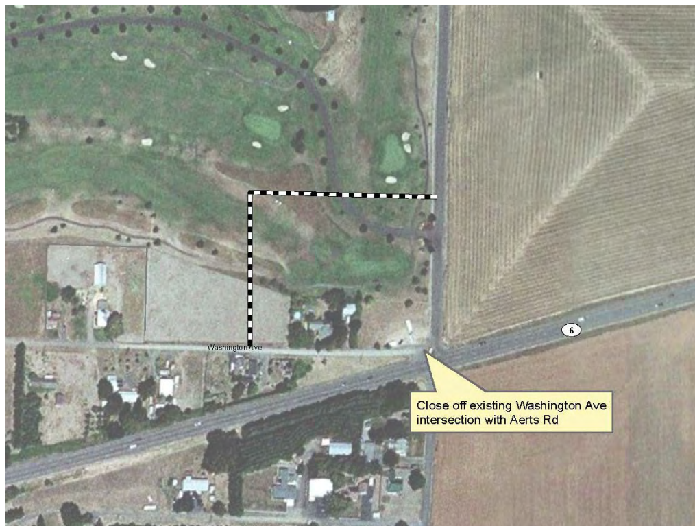
Figure 2: Alternative #2 - Realignment of Washington Avenue
