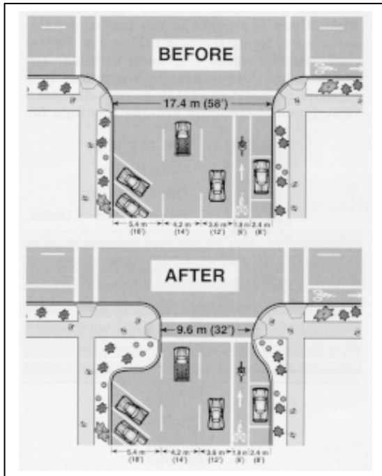
Figure 21. Example of curb extension Retrofit
