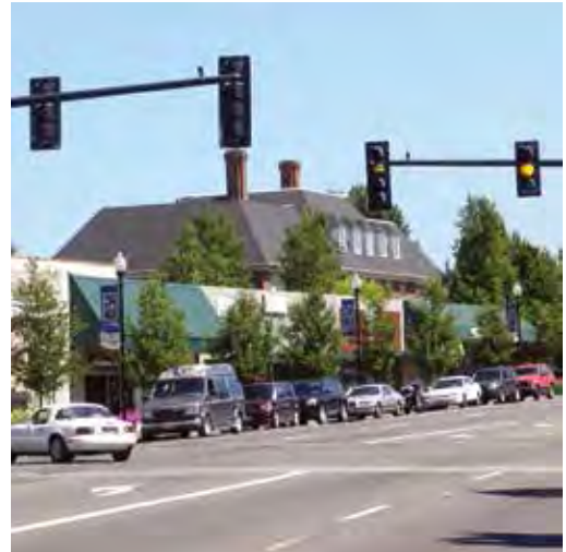
The intersection of E. Powell Boulevard at N. Main Avenue features flashing yellow arrow left-turn phasing.
