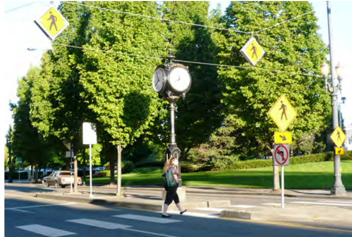
Overhead and roadside signs provide increased visibility for the presence of midblock crossings and indicate where pedestrians should cross. A pedestrian refuge allows pedestrians to cross one direction of the street at a time.
