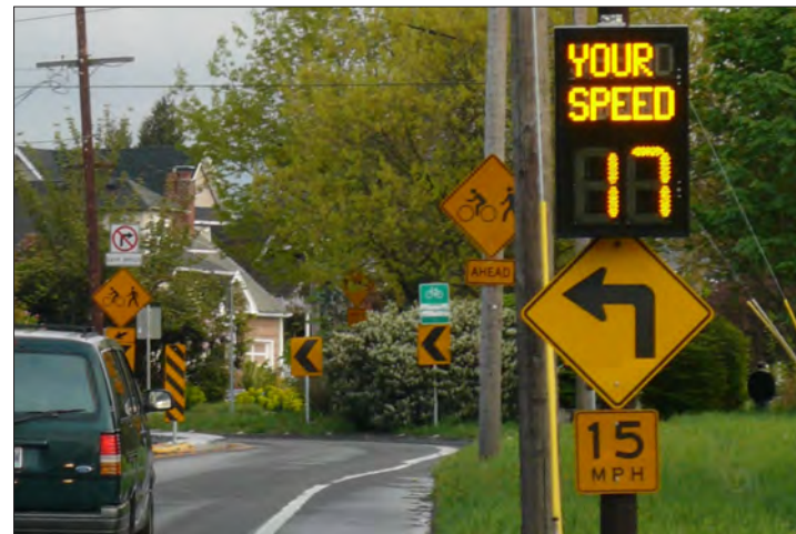
Active speed radar signs measure the speed of approach vehicles and are typically posted near cautionary or posted speed limits.
