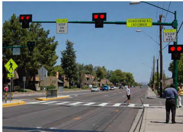
A H.A.W.K. signal is shown—High-intensity activated walk signal. These pedestrian activated street crossings couple signage, striping, and lighting to bring auto traffic to a stop so pedestrians can cross safely.
