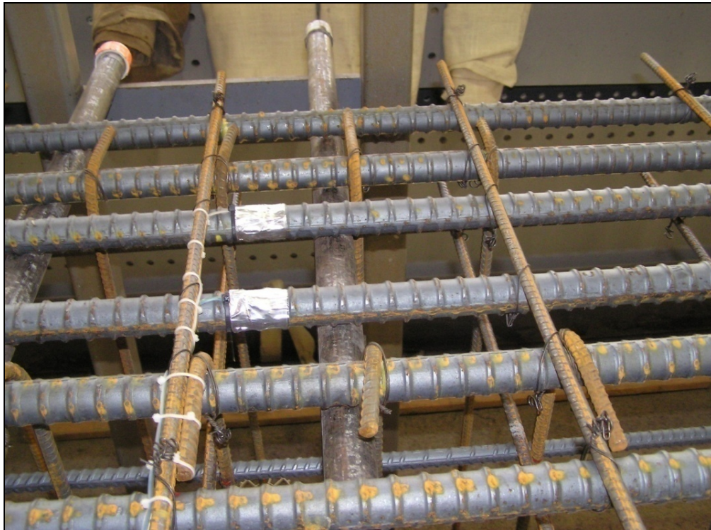
Figure 4.7: Typical strain gage locations along flexural steel
