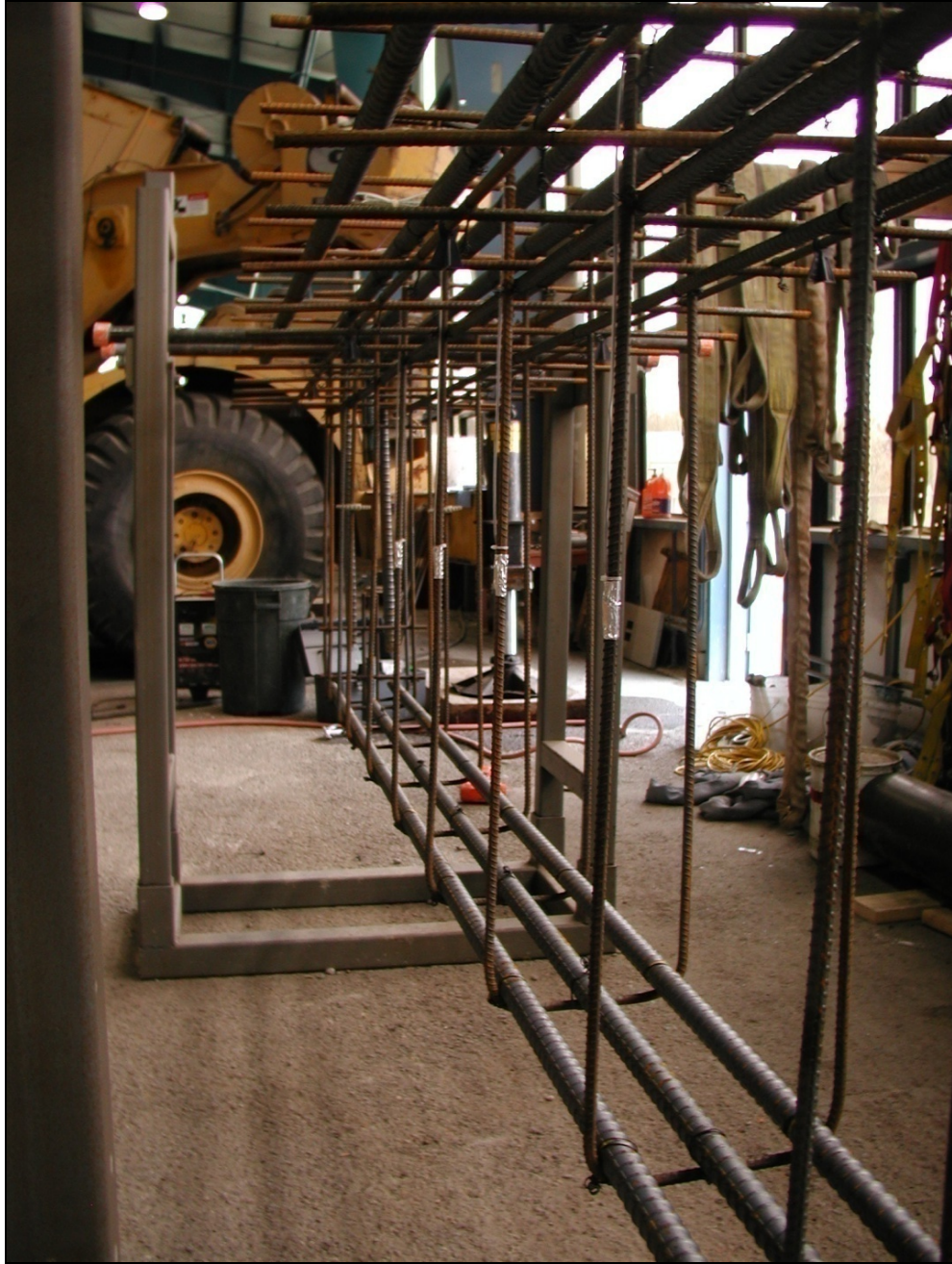
Figure 4.8: Typical strain gage locations along stirrups
