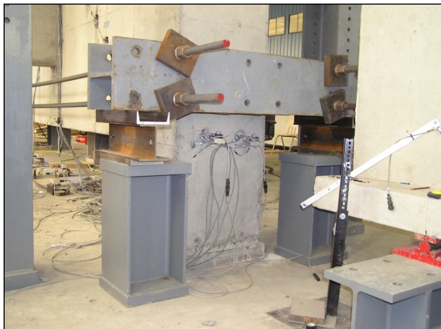
Figure 5.110: Post-tensioned bent cap installation: adjacent reaction beam
