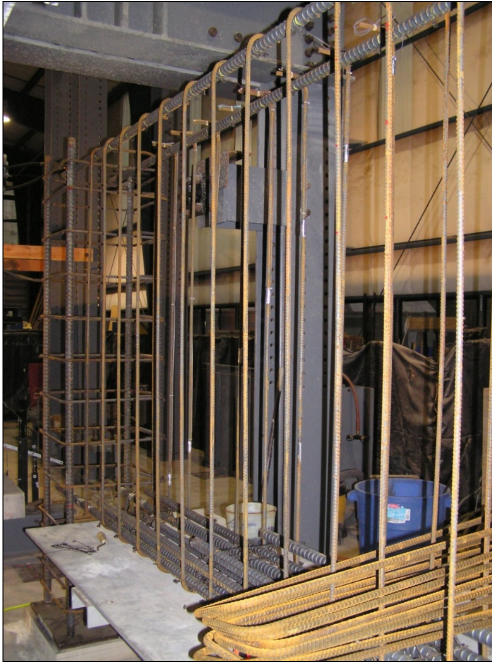
Figure 4.11: Typical bent cap stirrup assembly
