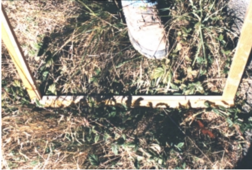
Example 3: Measurement shows 23cm of broadleaf, 11cm high, representing 51% coverage. Note dried dead grass that is not included in the measurement. Reference: site 3, MP29.11 + 100S on 10/12/99.
