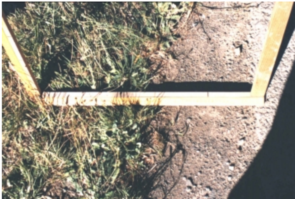
Example 4: Measurement shows 5cm of grass (11cm high) and 19 cm broadleaf (5cm high), representing 53% coverage. Note first 15 cm on right near road is not measured. Reference: site 3, MP29.51 + 140S on 10/12/99.
