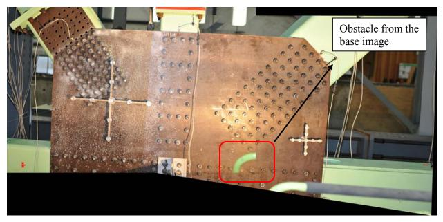
Figure 4.6: Stitched image with obstacle contained in the base image (Image 1). A polygon area including the obstruction is selected and the user can replace that area with part from Image 2
