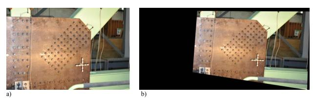
Figure 4.2: Transformed image (Image 2) a) Original base image and b) Boundaries of composite image populated with Image 2
