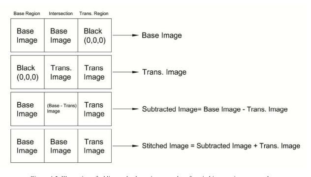
Figure 4.5: Illustration of adding and subtracting procedure for stitching two images together.
