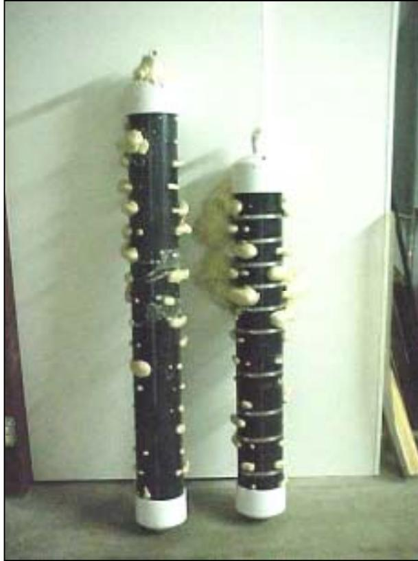
Figure 4.5: Penetration tubes after injection
