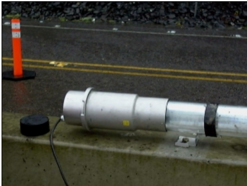
Figure 1.2: Light Injector at the End of a Section of Lighted Guidance Tube
