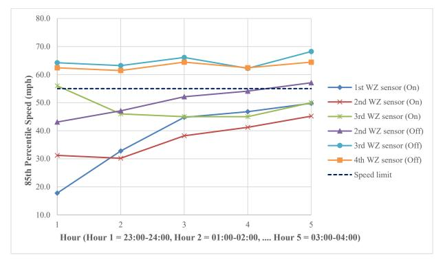
Figure 5.4: Hourly vehicle speed (85% percentile) at active WZ sensors for day 1 (blue lights on) and day 2 (blue lights off) (Case Study 1)
