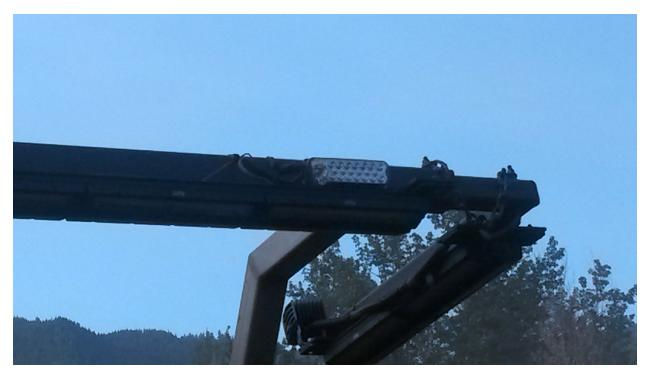
Figure 4.2: Blue light installed on paving equipment
