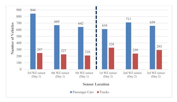
Figure 5.6: Traffic volumes for different vehicle types recorded by active WZ sensors for day 1 (blue lights off) and day 2 (blue lights on) (Case Study 2)
