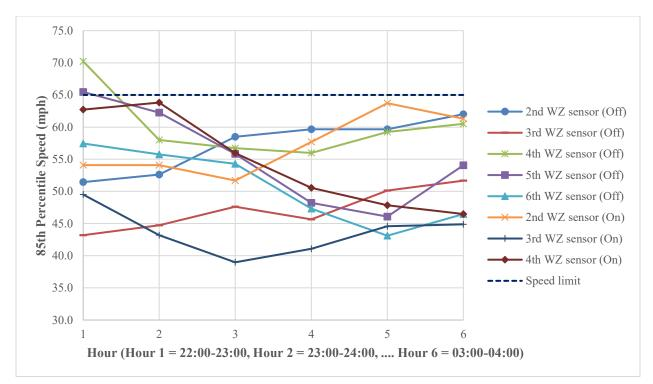
Figure 5.10: Hourly vehicle speed (85% percentile) at active WZ sensors for day 3 (blue lights off) and day 4 (blue lights on) (Case Study 2)
