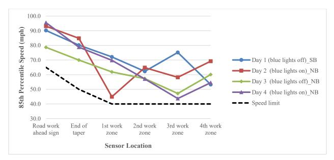
Figure 5.8: Vehicle speed (85th percentile) at different locations for all 4 days (Case Study 2)
