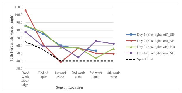
Figure 5.13: Vehicle speed (85th percentile) at different locations for all four days (Case Study 3)
