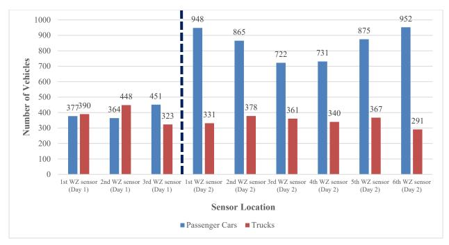
Figure 5.11: Traffic volumes for different vehicle types recorded by active WZ sensors for day1 (blue lights off) and day 2 (blue lights on) (Case Study 3)
