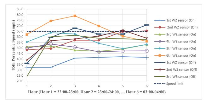
Figure 5.14: Hourly vehicle speed (85% percentile) at active WZ sensors for day 1 (blue lights off) and day 2 (blue lights on) (Case Study 3)
