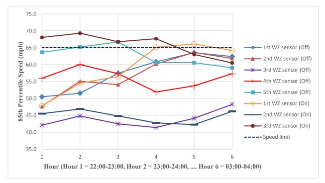
Figure 5.15: Hourly vehicle speed (85% percentile) at active WZ sensors for day 3 (blue lights off) and day 4 (blue lights on) (Case Study 3)
