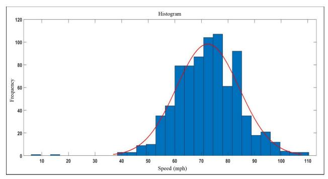
Figure 5.27: Histogram from sensor data at road work ahead sign (Case Study 2)
