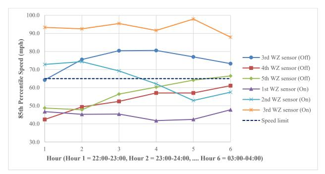
Figure 5.9: Hourly vehicle speed (85% percentile) at active WZ sensors for day 1 (blue lights off) and day 2 (blue lights on) (Case Study 2)
