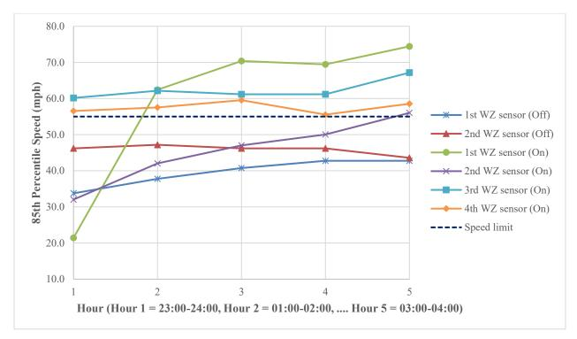
Figure 5.5: Hourly vehicle speed (85% percentile) at active WZ sensors for day 3 (blue lights off) and day 4 (blue lights on) (Case Study #1)
