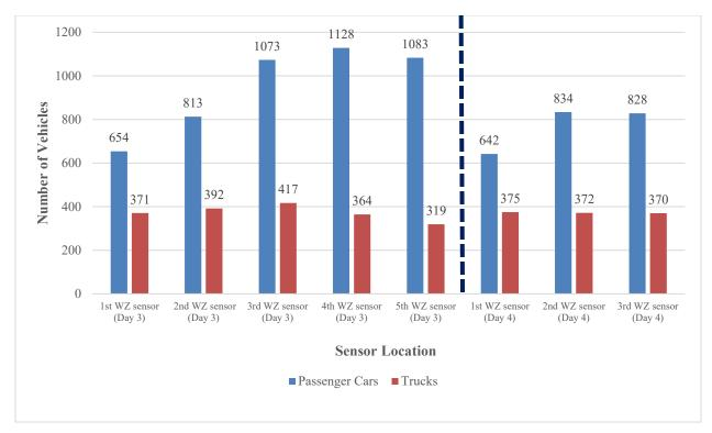
Figure 5.12: Traffic volumes for different vehicle types recorded by active WZ sensors for day 3 (blue lights off) and day 4 (blue lights on) (Case Study 3)
