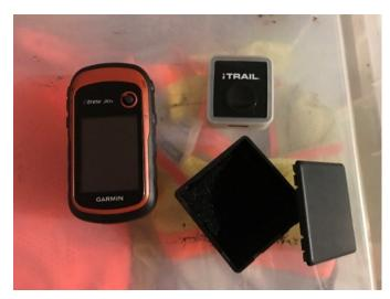
Figure 3.6: Handheld GPS device (left), and GPS tracker and casing for GPS tracker (right)
