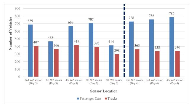
Figure 5.7: Traffic volumes for different vehicle types recorded by active WZ sensors for day 3 (blue lights off) and day 4 (blue lights on) (Case Study 2)
