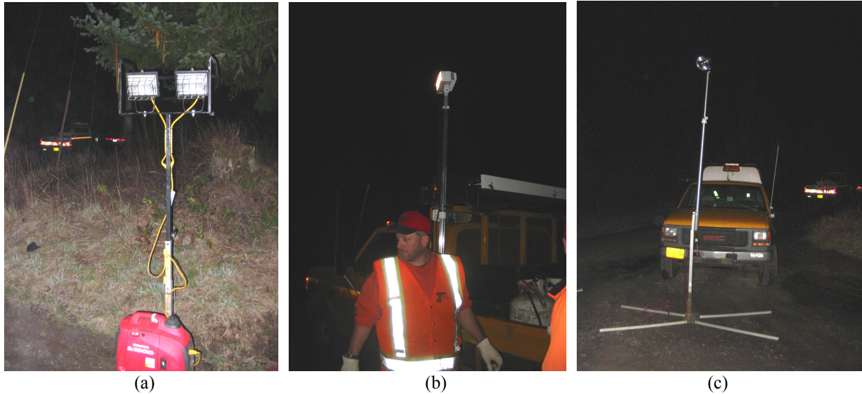
Figure 3.1: Typical lights used by ODOT Maintenance: (a) 6-foot tall, dual luminaire with portable generator; (b) single luminaire mounted on truck; and (c) single spotlight mounted on tripod
