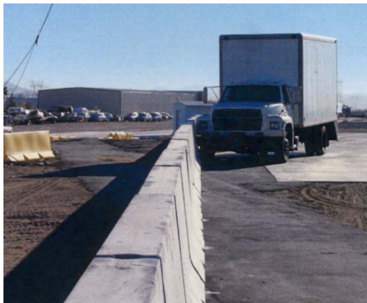
Figure 3.5: Test vehicle prior to Crash Test 3, showing angle of impact
