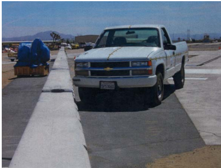
Figure 3.3: Test vehicle prior to Crash Test 2, showing angle of impact
