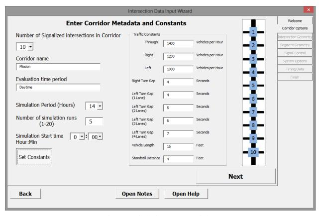
Figure 8.3: Simulation Constants Window
