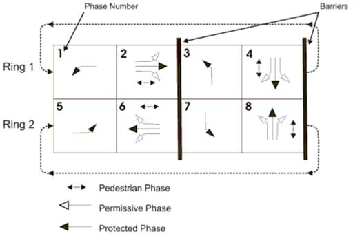
Figure 6.1: NEMA Phasing Diagram (FHWA 2012)
