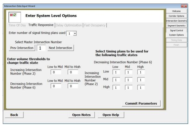
Figure 8.12: System Level Parameters – Traffic Responsive
