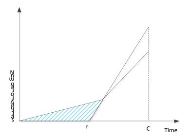
Figure 5.2: Arrival and Departure Queuing Diagram for a Coordinated Intersection
