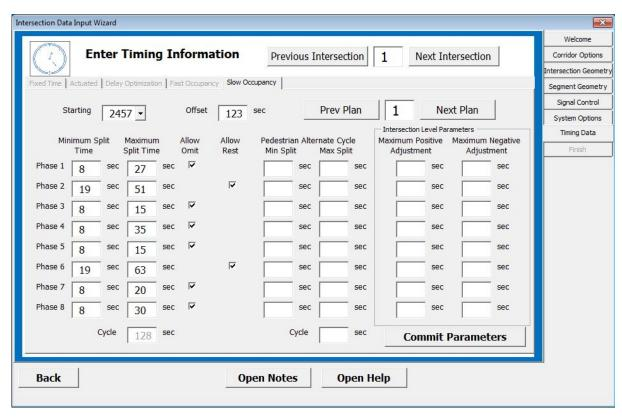
Figure 8.16: Signal Timing Information Entry - Faux ACS Lite
