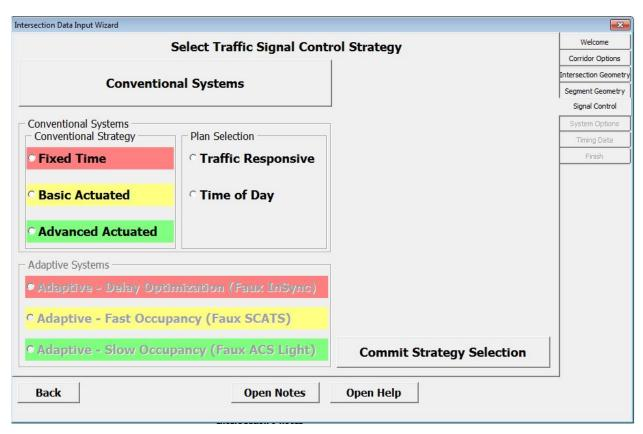
Figure 8.8: Traffic Signal Control System Selection
