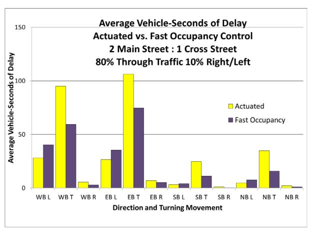
Figure 4.4: Vehicle-Seconds of Delay for Actuated Control vs. Fast Occupancy Algorithm Under Platooned Arrivals
