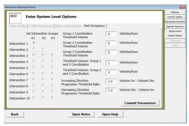
Figure 8.9: System Level Parameters – Faux SCATS
