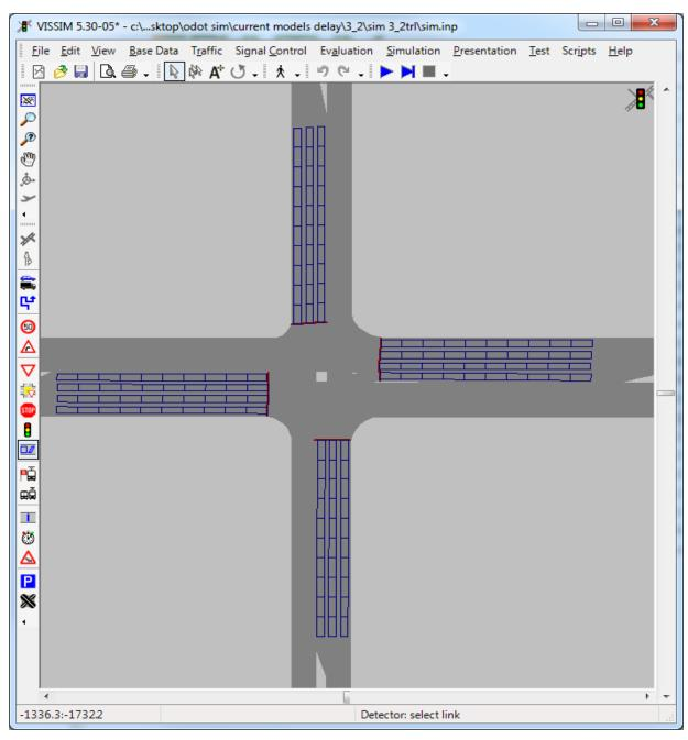
Figure 4.2: Detector Placement for Delay Optimization Strategy
