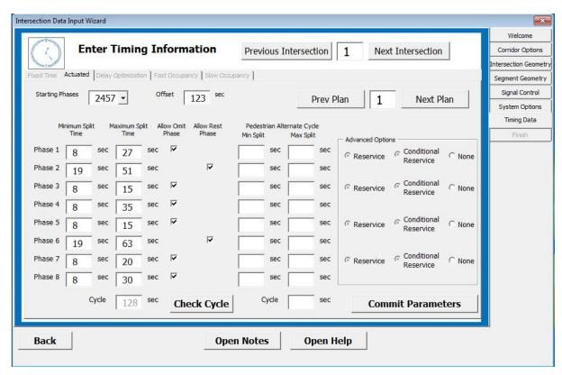
Figure 8.17: Signal Timing Information Entry – Actuated Control
