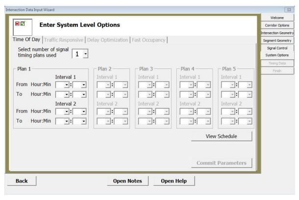
Figure 8.11: System Level Parameters – Time of Day plan selection
