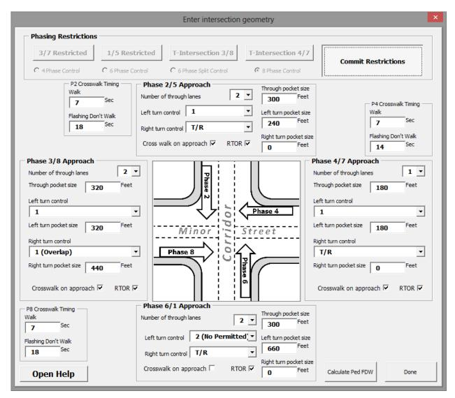
Figure 8.6: Intersection Geometry with Phasing Restrictions Committed
