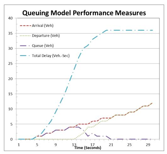
Figure 5.3: Arrival and Departure Diagram for Discreet Time Intervals with Queue Length and Total Delay
