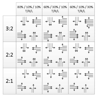
Figure 4.1: Lane Configurations by Approach Configuration and Turning Movement Bias
