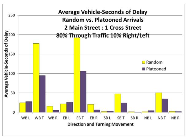
Figure 4.3: Average Vehicle-Seconds of Delay by Movement at 2:1 Intersection Under Actuated Control with 600:300 vphpl Input Volumes
