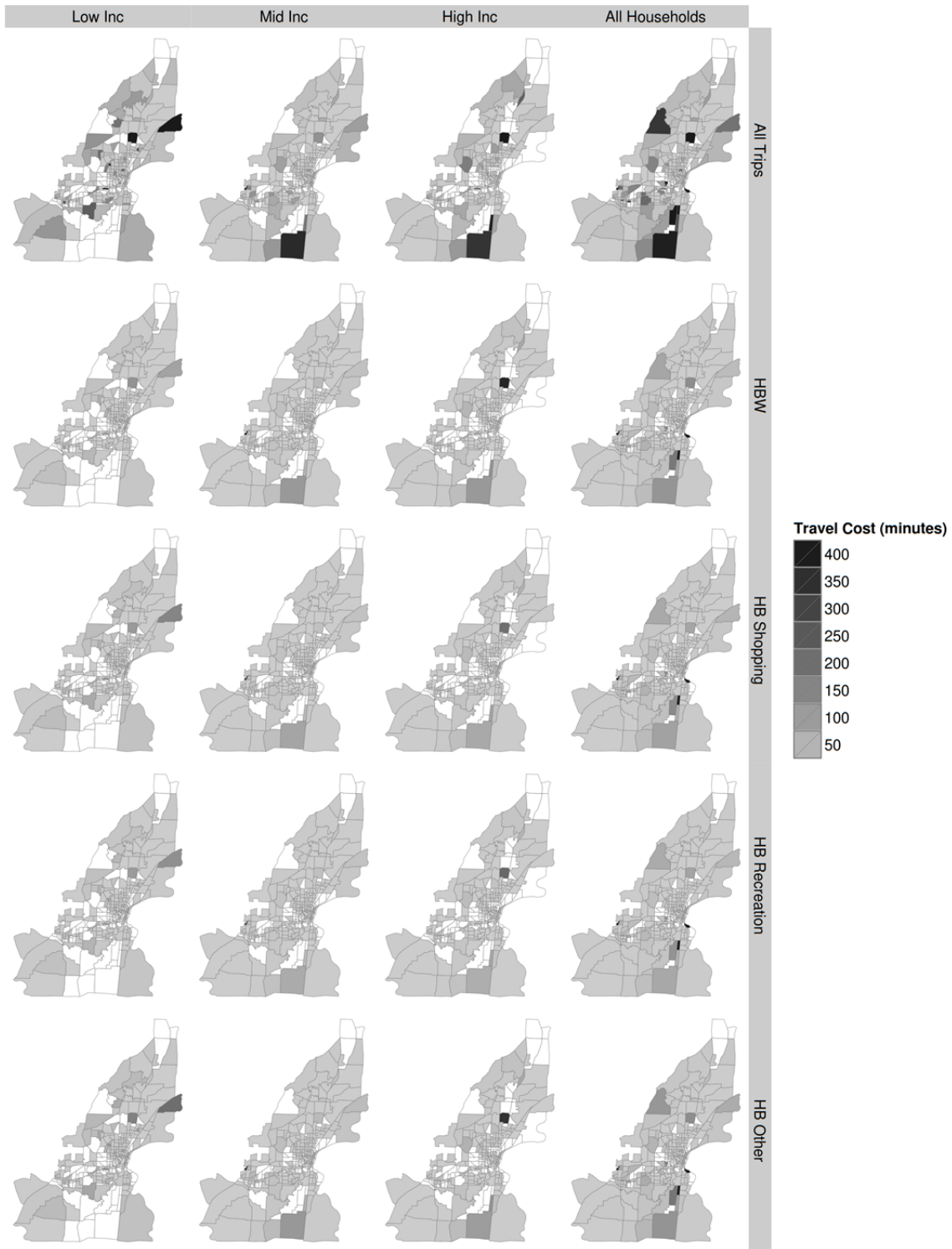
Figure 6.10: TAZ level travel costs by income level and trip purpose for Corvallis Scenario A (halving auto travel time; all other data from the 2010 CAMPO JEMnR model)
