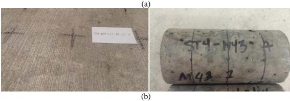
Figure 4.16: (a) Surface deterioration in ST2 slabs (without air entrainment) after 60 F-T cycles, (b)ST4 slab and accompanying concrete cylinder after the completion of the F-T study.
