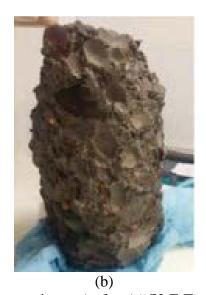
Figure 4.10: Deterioration in ST2 cylinders (without air entrainment) after (a) 72 F-T cycles, (b) 108 F-T cycles under ASTM C666 Procedure B protocol.
