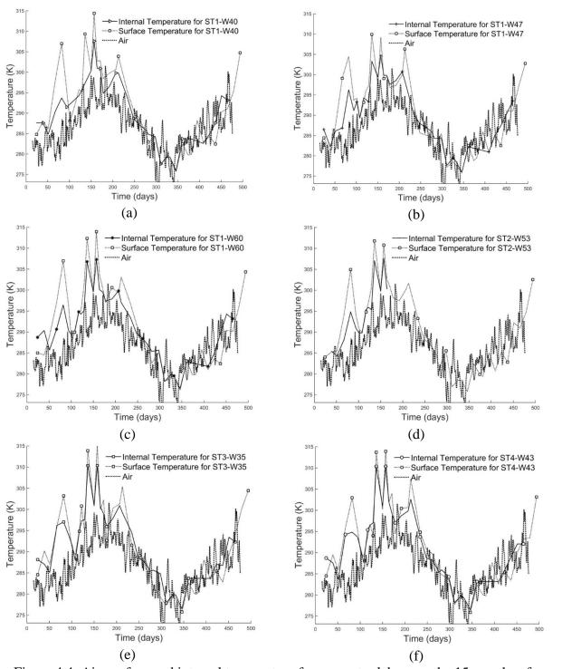
Figure 4.4: Air, surface and internal temperature for concrete slabs over the 15 months of chloride testing: (a) ST1-A, (b) ST1-B, (c) ST1-C, (d) is ST2, (e) ST3, and (f) ST4.
