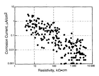
Figure 2.5: Inverse relationship between corrosion current and concrete resistivity from field measurements (*Carino 1999*).
