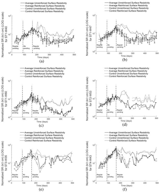
Figure 4.7: Surface resistivity measurements taken over the unreinforced section of the control slabs and the de-icing solution ponded slabs. (a) ST1-A, (b) ST1-B, (c) ST1-C, (d) is ST2, (e) ST3, and (f) ST4. Measurements are normalized for 77°F (25 °C).
