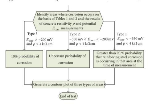
Figure 2.6: Suggested methodology when assessing four-point Wenner probe electrical resistivity and half-cell potential measurements (*Sadowski 2013*).
