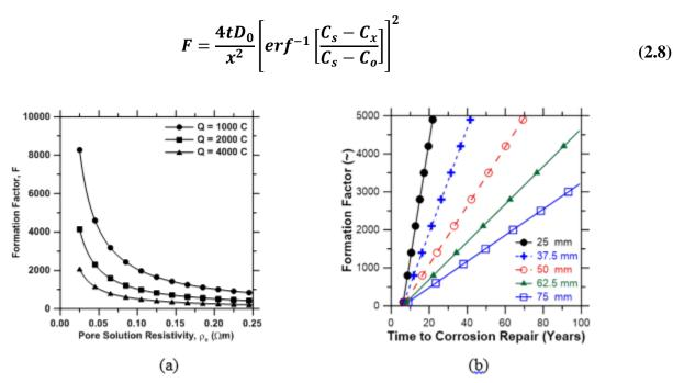
Figure 2.2: The relationship between (a) the RCP test and the formation factor for various pore solution resistivities, and (b) the predicted time to corrosion as a function of cover thickness (Weiss et al. 2016).
