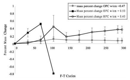
Figure 4.12: Percent mass change over time on cylinders that underwent 300 F-T cycles in the Scientempt chamber. Three types of concrete were tested: 1) OPC concrete with w/c ratio of 0.53 and no air-entrainment, 2) an OPC concrete w/cm ratio of 0.47 with air-entrainment and 3) a HPC with a w/cm ratio of 0.43 that contained silica fume, fly ash and air-entrainment.
