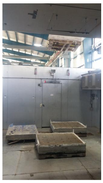
Figure 9-6: Reinforced concrete slabs in the F-T chamber.
