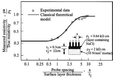
Figure 2.3: Normalized resistivity values over the ratio of probe spacing to surface layer thickness containing chlorides (*Gowers and Millard 1999*).
