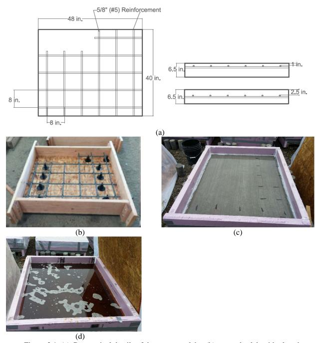
Figure 3.1: (a) Geometrical details of the concrete slabs; (b) a sample slab with placed reinforcement before casting of concrete; (c) a completed slab ready for ponding; (d) a sample concrete slab during ponding with the deicing solution. The section that is unreinforced was used to take measurements and to extract cores for additional testing.
