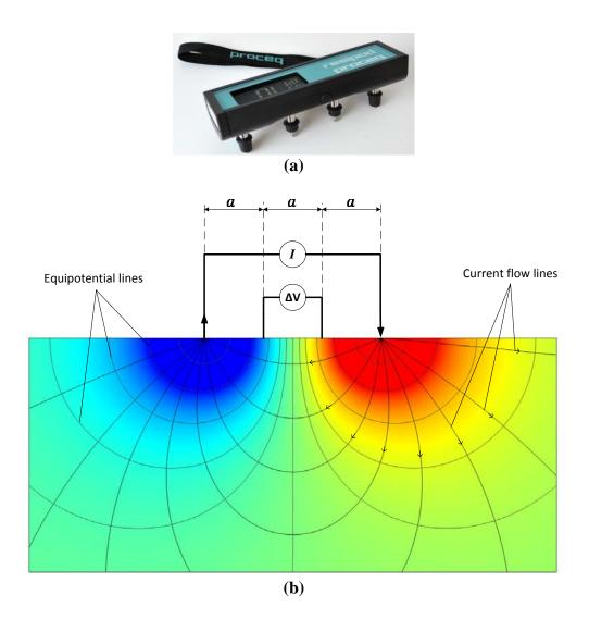
Figure 2.1: (a) A commercial Wenner probe (*Proceq 2011*); (b) functional schematic of the probe (*Salehi 2013*).
