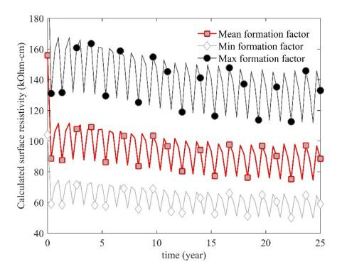
Figure 6.6: Effects of formation factor coefficient, m, on SR over bridge deck age. The considered values for m were 1.8, 2.0, and 2.2 for min, mean and max values, respectively.
