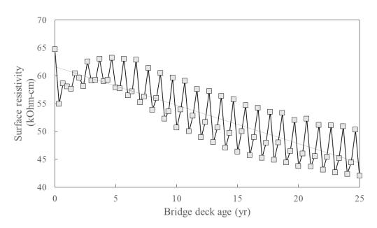
Figure 6.4: SR predictions of the example case over time (not normalized for temperature).
