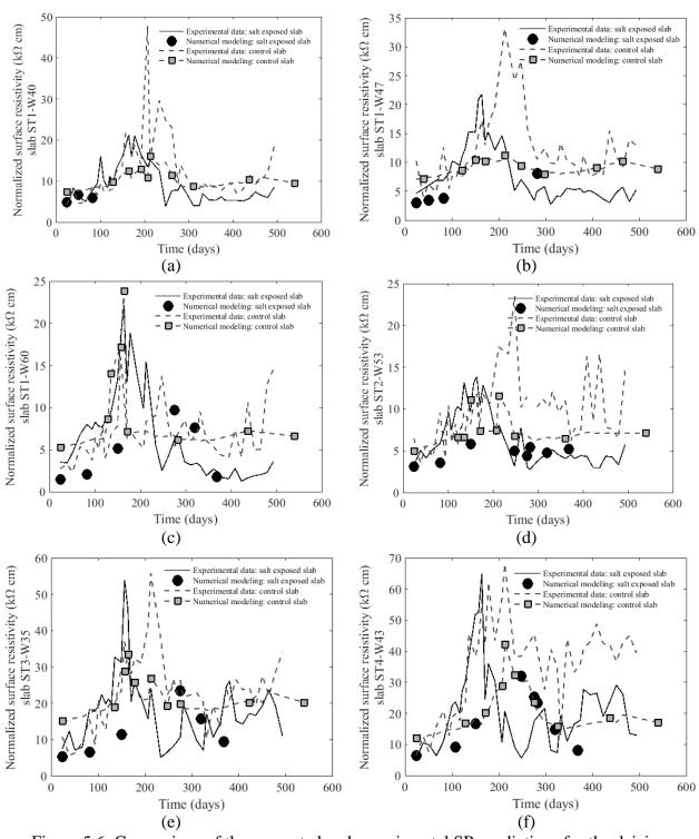
Figure 5.6: Comparison of the computed and experimental SR predictions for the deicing chemical exposed and water exposed slabs (a) ST1-W40, (b) ST1-W47, (c) ST1-W60, (d) ST2-W53, (e) ST3-W35 and (f) ST4-W43.
