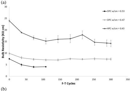
Figure 4.9: Surface (a) and bulk (b) resistivity taken on cylinders that underwent 300 F-T cycles according to ASTM C666 Procedure B. Three types of concrete were tested: 1) OPC concrete with w/c ratio of 0.53 and no air-entrainment (ST 2) an OPC concrete w/cm ratio of 0.47 with air-entrainment (ST1-C) and 3) a HPC with a w/cm ratio of 0.43 that contained silica fume, fly ash and air-entrainment (ST4). Measurements are normalized for 77°F (25 °C).
