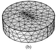
Figure 5.4: (a) Domain geometry with the Wenner probe locations on top; (b) FEM discretization.
