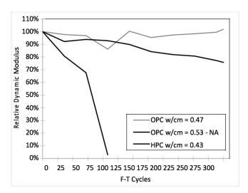
Figure 4.13: Relative dynamic modulus of elasticity on concrete cylinders after 300 F-T cycles in the in the Scientempt chamber.
