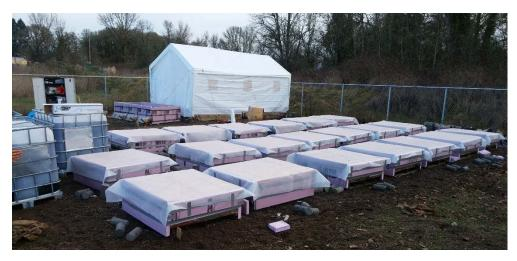
Figure 9-4: Slabs in ponding cycle at the OSU outdoor exposure site. Deicer containers can be seen at the far end.
