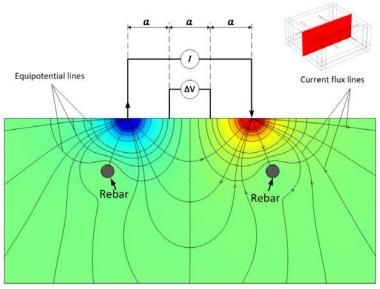
Figure 5.2: Typical configuration of Wenner probe resistivity measurement in reinforced concrete (*Salehi et al. 2016*).
