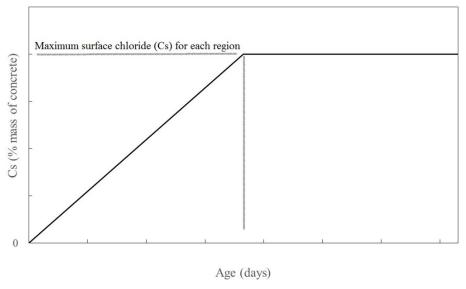
Figure 5.3: The boundary condition for salt on bridge deck surface.
