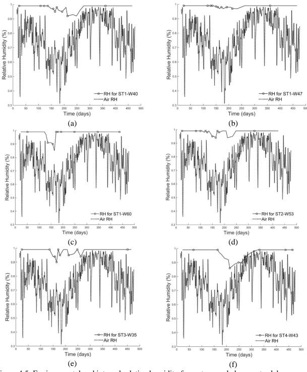
Figure 4.5: Environmental and internal relative humidity for water-ponded concrete slabs over the 15 months of chloride testing: (a) ST1-A, (b) ST1-B, (c) ST1-C, (d) is ST2, (e) ST3, and (f) ST4.
