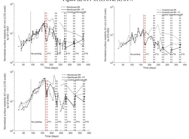
Figure 4.15: Surface resistivity measurements taken on reinforced slabs throughout 28 ponding cycles. Each D-T cycles is shown with vertical doted lines labeled FT1, FT2, FT3, etc. Figure (a) ST1-C, (b) ST2, (c) ST4.
