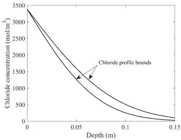
Figure 6.8: Chloride profiles at the time of the inspection (10 years from casting) for the demonstration study example for a hypothetical bridge near Bend, Oregon.
