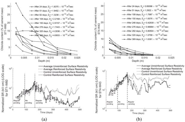
Figure 4.8: The effect of chloride ingress on SR measurements (a) ST1 slab with w/cm 0.60, (b) ST4 slab with w/cm 0.43.
