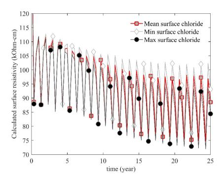
Figure 6.7: Effects of surface chloride concentration uncertainties on SR over bridge deck age. The surface chloride concertation was assumed to have  $\pm 20\%$  uncertainty over the average values.
