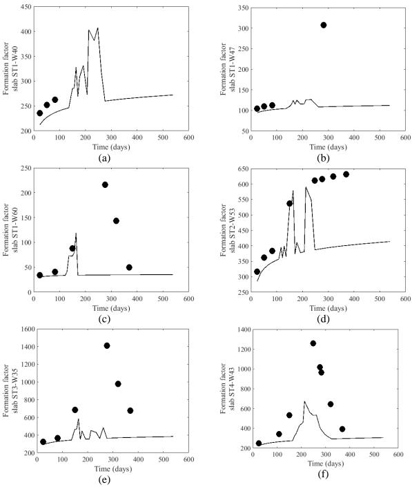
Figure 5.5: Comparison of the computed formation factors for the deicing chemical exposed and water exposed slabs (a) ST1-W40, (b) ST1-W47, (c) ST1-W60, (d) ST2-W53, (e) ST3-W35 and (f) ST4-W43.
