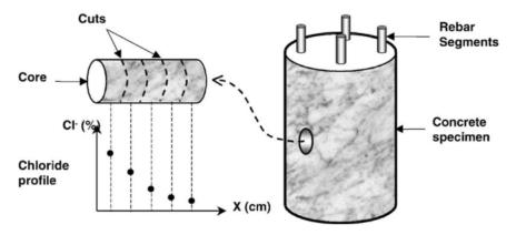
Figure 2.4: Reinforced concrete specimen geometry and chloride profile sample selection (*Morris et al. 2004*).
