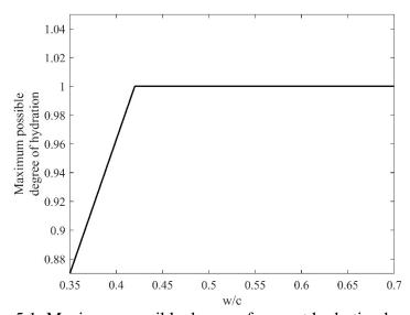
Figure 5.1: Maximum possible degree of cement hydration based on w/c.
