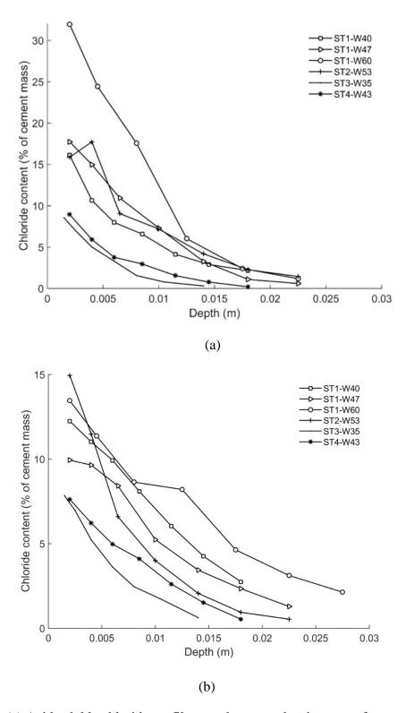
Figure 4.1: (a) Acid soluble chloride profiles are shown on the six types of concrete after (a) 14 ponding cycles; (b) 20 ponding cycles. ST1-W40 had a w/c ratio of 0.40, ST1 -W47 had a w/c ratio of 0.47, ST1-W60 had a w/c ratio of 0.60, ST2-W53 had a w/c ratio of 0.53, ST3 had a w/c ratio of 0.35 and ST4 had a w/c ratio of 0.43.
