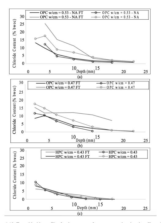
Figure 4.18: Two chloride profiles for three types of concrete are showing the effect of F-T action on chloride ingress. An OPC concrete with w/c ratio of 0.53 and no air-entrainment, an OPC concrete w/cm ratio of 0.47 with air-entrainment and a HPC with a w/cm ratio of 0.43.
