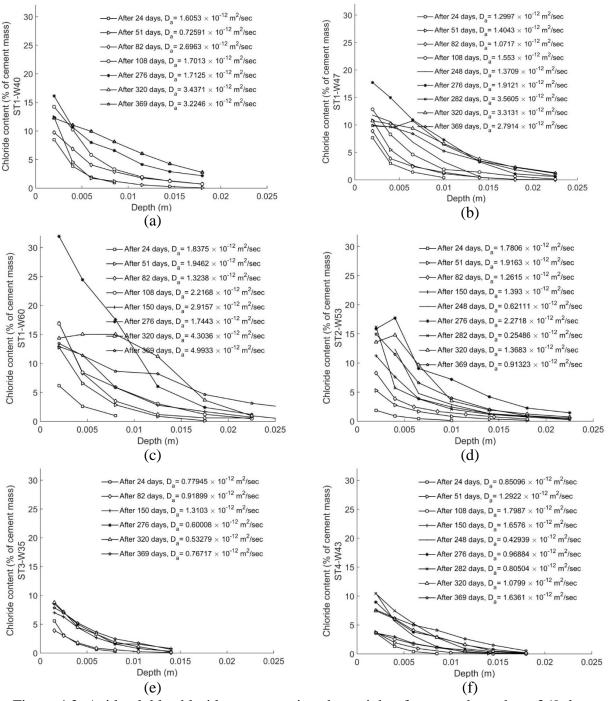
Figure 4.2: Acid-soluble chloride concentrations by weight of cement throughout 369 days of cyclic ponding with their respective apparent diffusion coefficients. (a) is ST1 with w/c ratio of 0.40, (b) is ST1 with w/c ratio of 0.47, (c) is ST1 with w/c ratio of 0.60, (d) is ST2 with w/c ratio of 0.53, (e) is ST3 with w/c ratio of 0.35 and (f) is ST4 with w/c ratio of 0.43.
