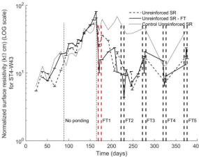
Figure 4.14: Surface resistivity measurements taken on unreinforced slabs throughout 28 ponding cycles. Each D-T cycles is shown with vertical doted lines labeled FT1, FT2, FT3, etc. Figure (a) ST1-C, (b) ST2, (c) ST4.
