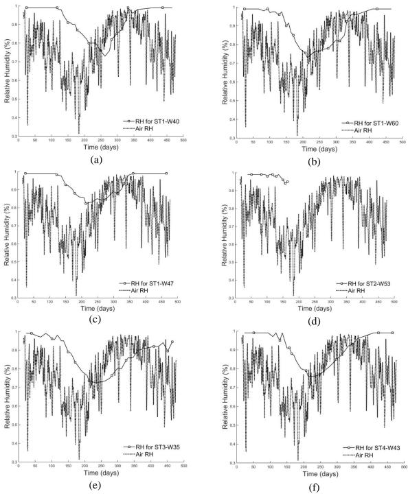
Figure 4.6: Environmental and internal relative humidity for de-icing solution-ponded concrete slabs over the 15 months of chloride testing: (a) ST1-A, (b) ST1-B, (c) ST1-C, (d) is ST2, (e) ST3, and (f) ST4.
