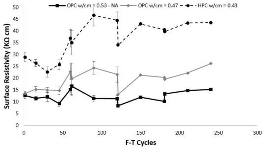
Figure 4.17: Surface resistivity taken on cylinders that underwent two sets of 60 F-T cycles in a controlled environmental chamber. An OPC concrete with w/c ratio of 0.53 and no airentrainment, an OPC concrete w/cm ratio of 0.47 with air-entrainment and a HPC with a w/cm ratio of 0.43 that contained silica fume, fly ash and air-entrainment.
