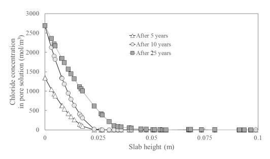
Figure 6.3: Chloride profiles of the example case over bridge deck thickness after 5, 10 and 25 years of exposure.
