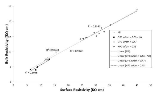
Figure 4.11: Linear regression relationship between SR and bulk resistivity taken on cylinders for each type of concrete.
