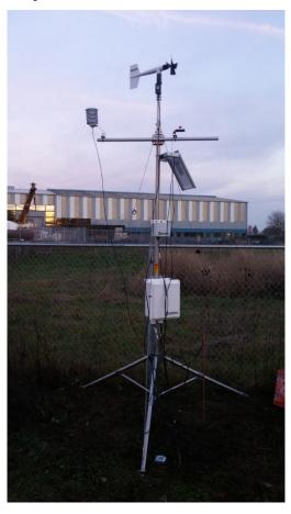
Figure 9-5: Installed weather station at the OSU outdoor exposure site.
