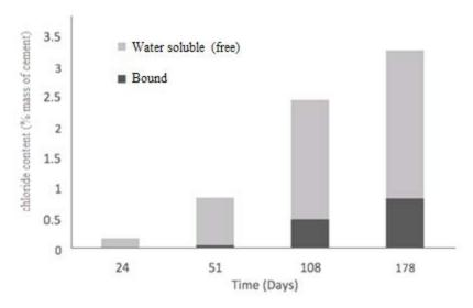
Figure 4.3: Free and bound chloride concentration of ST2 at 10 mm in depth over time.
