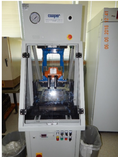
Figure 3.7: Laboratory Compaction; (a) Superpave Gyrotory Compactor and cylindrical specimens; (b) Roller Compactor and beam specimens
