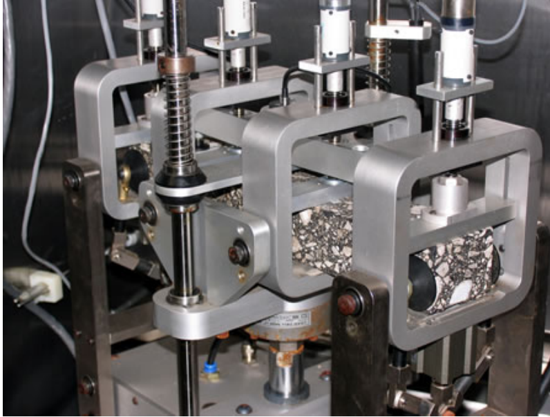
Figure 2.7: Four-point bend testing system (Source: www.pavementinteractive.org ).
