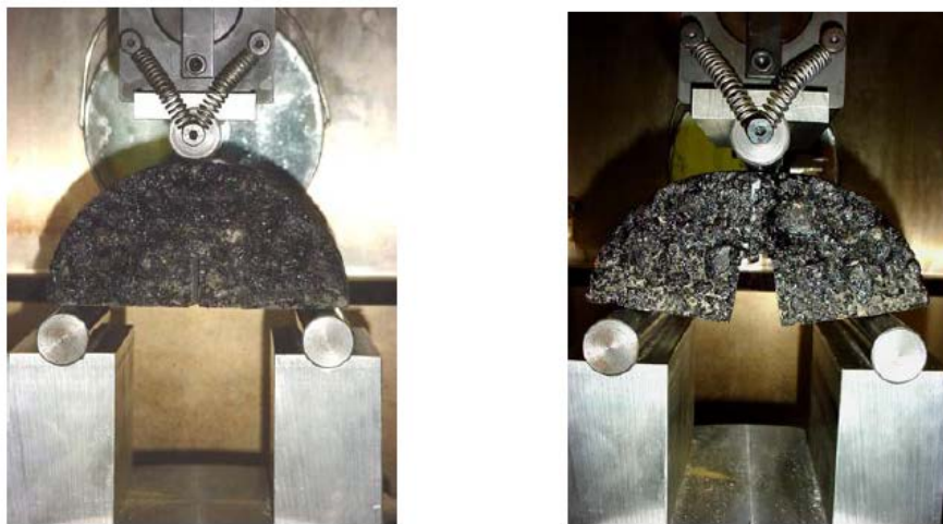
Figure 2.11: SCB test apparatus (Wu et al. 2005).
