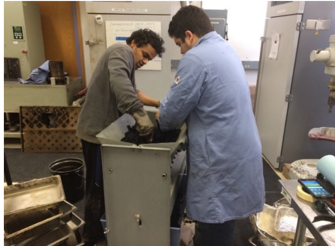
Figure 3.5: Mechanical Splitting of Asphalt Mixtures
