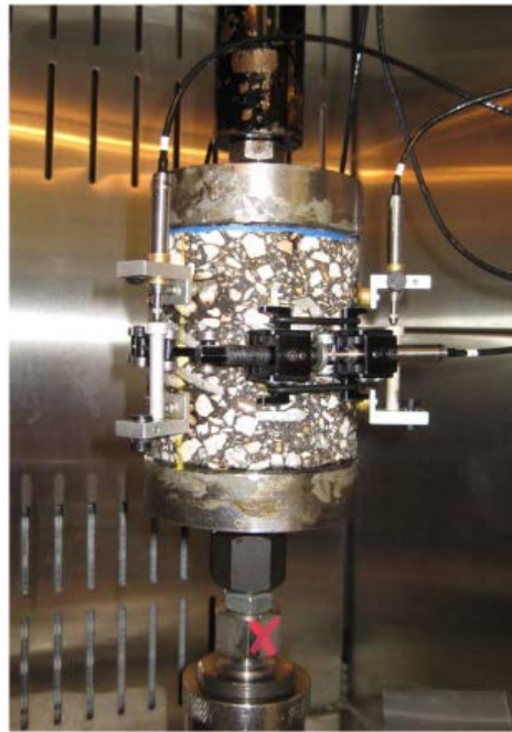
Figure 2.9: Configuration of controlled-strain RDT test (Luo et al. 2013).
