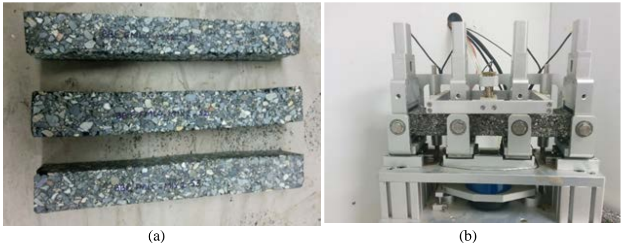
Figure 3.14: Bending beam fatigue test; (a) Beam specimens prepared with roller compactor; (b) four-point bending test apparatus
