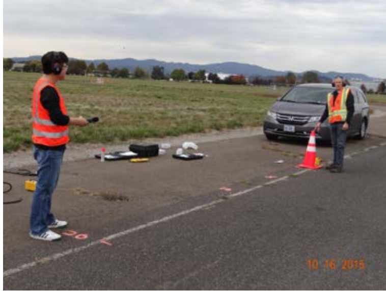
Figure 5.4: Sound Measurement at 20 feet
