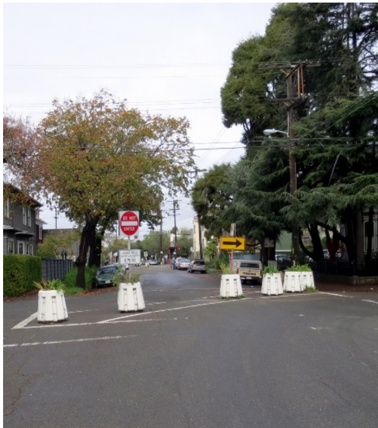
Figure 5.29: Bollards used to keep vehicles from entering, (N/A, N/A)
