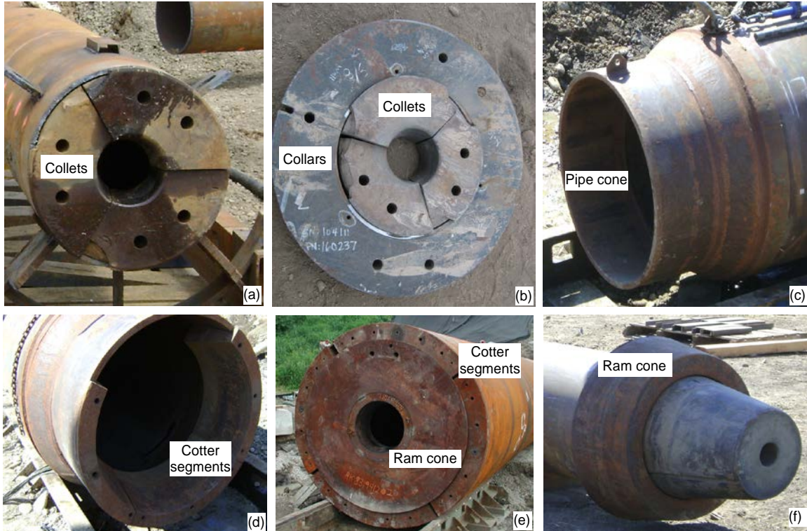
Figure 7.9: Hammer-pipe connections (a) collets showing moderate wear or damage (b) pipe ram collar and collets, the latter showing significant wear (c) pipe reducing cone/adaptor, and (d) cotter segments (e) ram cone and cotter segments, and (f) ram cone.
