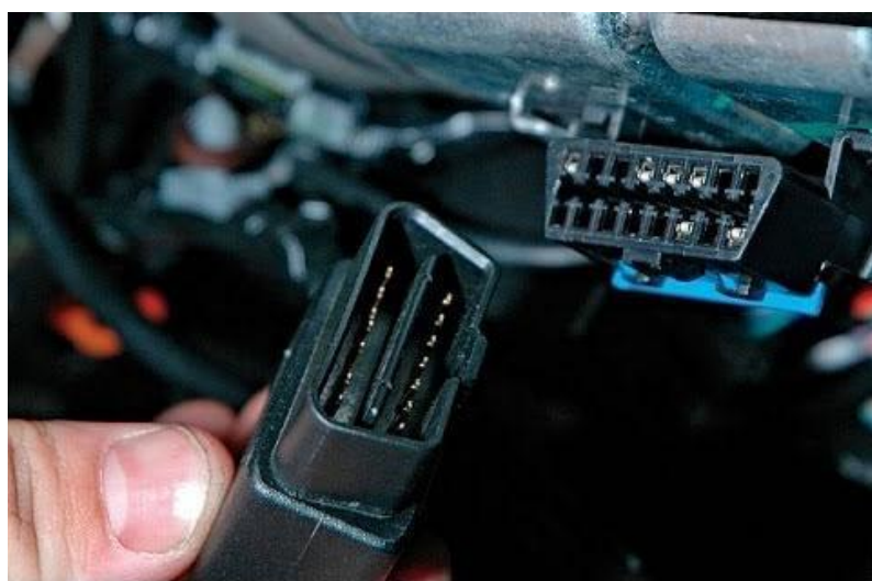
Figure 3: A GPS tracker plugs directly into the vehicle's OBD port. 15
