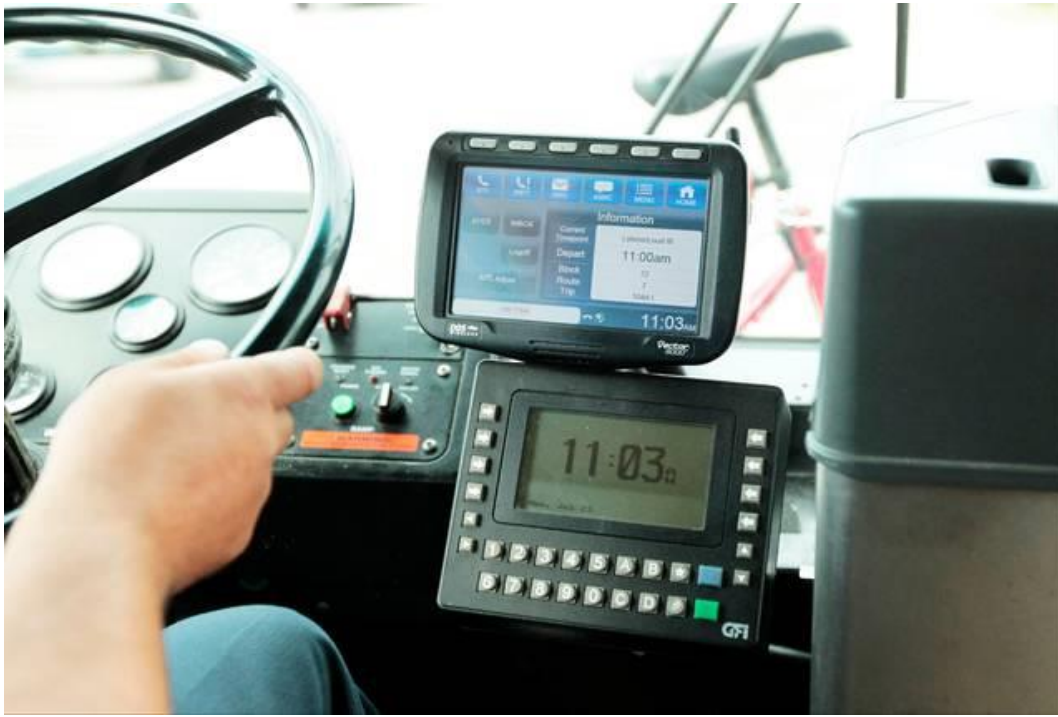
Figure 4: A Lextran bus' mobile data terminal, top, serves as a GPS device and receives information from the dispatch center and the control panel for the electronic farebox. 21
